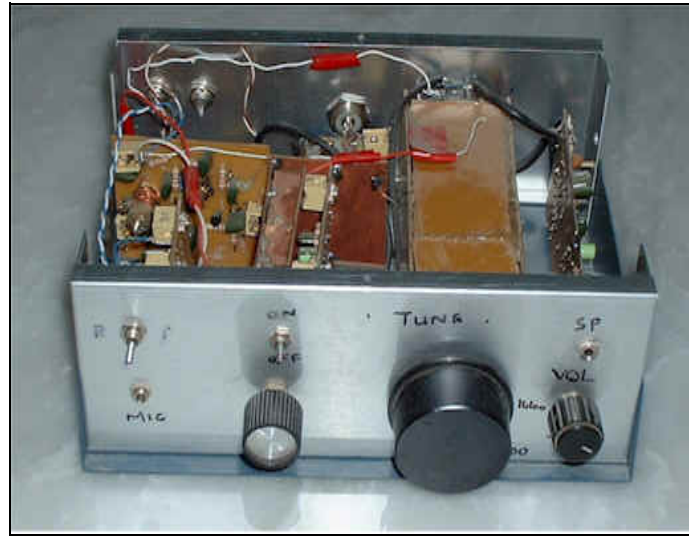
St2nh's homebrew DSB 20 m Radio 0.5 watts
