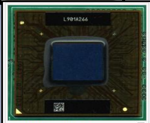
Pentium II: example of an interposer, integrated circuit die to ball grid array chip carrier
