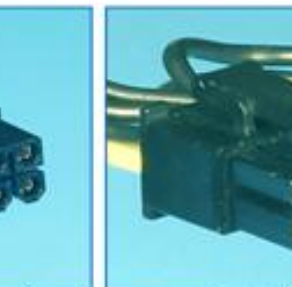
6+2 pin PCI Express power cable
