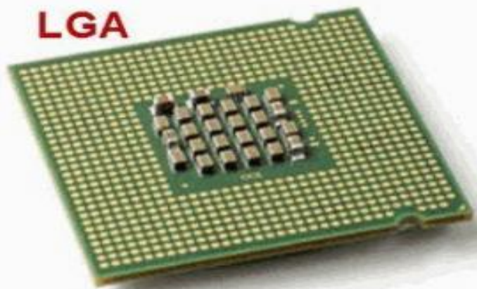
The LGA 775 socket on a Pentium 4 Prescott CPU. www.hasa.ps
