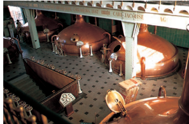
Figure 41.21 Beer Fermentation. Beer making can be carried out on a large scale or in the kitchen. In large-scale processes, copper brewing vats are often used, as shown here in the Carlsberg Brewery, Copenhagen, Denmark.
