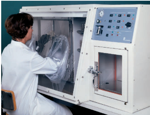
Figure 6.15 An Anaerobic Work Chamber and Incubator. This anaerobic system contains an oxygen-free work area and an incubator. The interchange compartment on the right of the work area allows materials to be transferred inside without exposing the interior to oxygen. The anaerobic atmosphere is maintained largely with a vacuum pump and nitrogen purges. The remaining oxygen is removed by a palladium catalyst and hydrogen. The oxygen reacts with hydrogen to form water, which is absorbed by desiccant.
