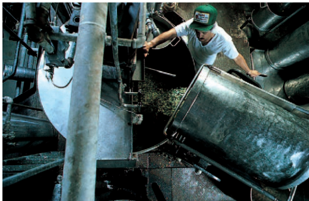
Figure 41.7 A Canning Operation. Microbial control is important in the processing and preservation of many foods. Worker pouring peas into a large, clean vat during the preparation of vegetable soup. After preparation the soup is transferred to cans. Each can is heated for a short period, sealed, processed at temperatures around 110–121°C in a canning retort to destroy spoilage microorganisms, and finally cooled.
