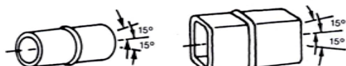
C—POSITION 5G PIPE OR TUBE HORIZONTAL FIXED ( \pm 15^\circ ). WELD FLAT, VERTICAL, OVERHEAD
