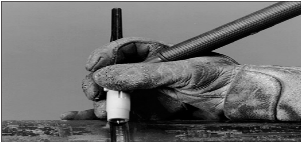
Figures 8.11 and 8.12 Demonstrations of two common methods of grasping the torch for pipe welding. There is no single "correct" method of doing this and each welder is encouraged to experiment with several different methods until one is found that is most comfortable, and results in satisfactory welds.
