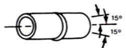
A—POSITION 1G PIPE HORIZONTAL AND ROTATED. WELD FLAT ( \pm 15^\circ ). DEPOSIT FILLER METAL AT OR NEAR THE TOP.
