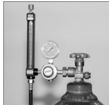
Figure 4.15 The regulator/flowmeter regulates the flow of shielding gas from the cylinder to the welding torch. This meter displays the amount of pressure in the cylinder as well as the rate of flow.
