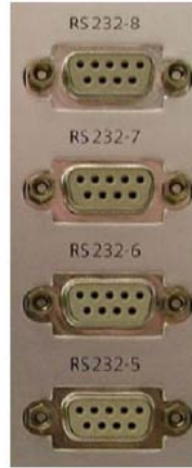
Figure 14: The RS232-5 up to 8 interface sockets of the PowerLink system
