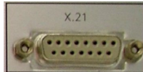
Figure 22: The X.21 interface socket of the PowerLink connector panel
