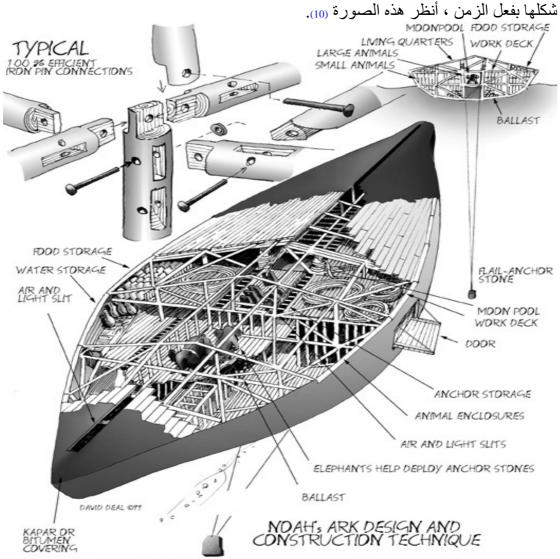
550 FOOT (22 INCH CUBIT) WOODEN VESSEL BUILT AS A FULLY TRIANGULATED TRUSS SPACE FRAME SKINNED WITH WOOD AND COVERED WITH BITUMEN OR TAR (CALLED KAPAR IN HEBREW)
