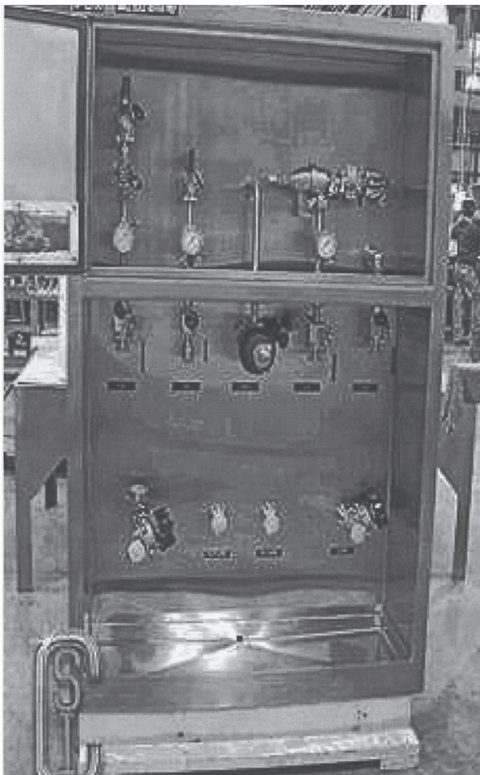
FIGURE 10 API Facility Hook-up Panel
